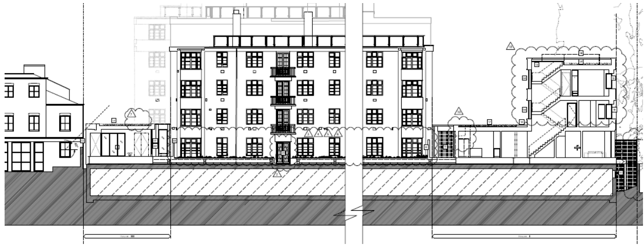
Section through Houses 2 & 3 showing William Court in the rear and Hamilton Garden properties to the right
